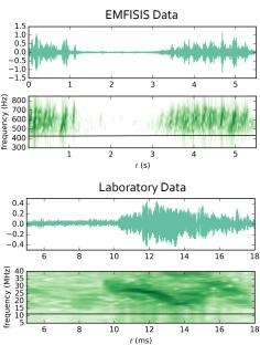
Figure 1: (Top) Bu component of Burst mode data taken from RBSP-B's EMFISIS instrument near a plasma boundary layer. Time series was recorded at 05:40:32.437892 UTC on 2012-11-14. (Bottom) Laboratory observation of Whistler Mode waves driven by plasma boundary layer. In both cases, electromagnetic waves are seen to be bursty with strong frequency chirping.
