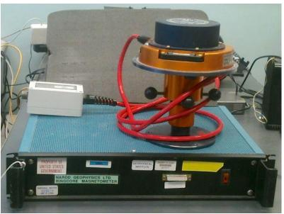
NAROD Three-axis fluxgate magnetometers Temperature stability: < 0.1 nT/degree (sensor);
