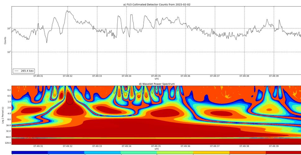
Top plot: An example of high resolution count data. Bottom Plot: Wavelet power spectrum from the above data. Statistically significant wavelet power from microbursts is enclosed by black contours in the high frequency region.
