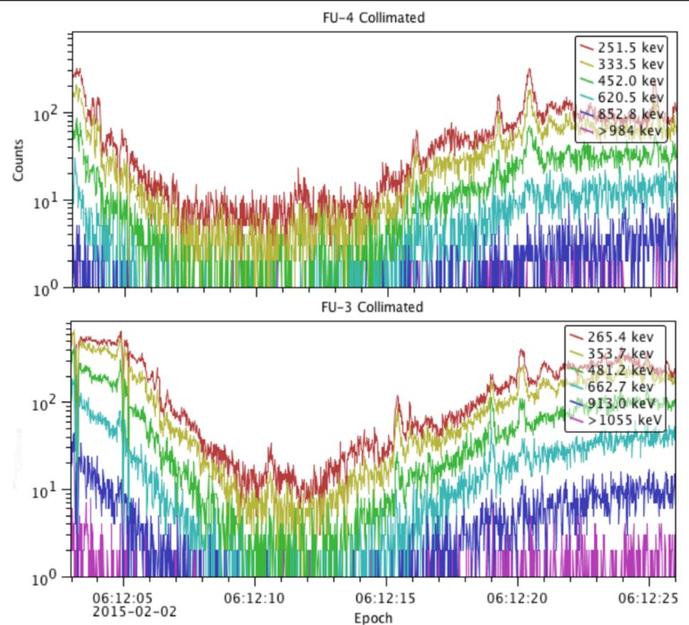
Visual inspection of microbursts on Feb 2<sup>nd</sup>, 2015 reveal two simultaneous bursts around 6:12:20 while both units were separated by 11 km. The automated wavelet-based microburst detection program will create a catalogue of these events from which microburst spatial and temporal properties can be decoupled [Alex Crew, 2016 JGR].
