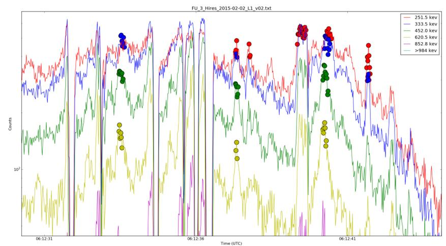
Microbursts detector applied to the six collimated energy channels on FU3. The detector has built in tests to avoid triggering on data gaps and dropouts.
