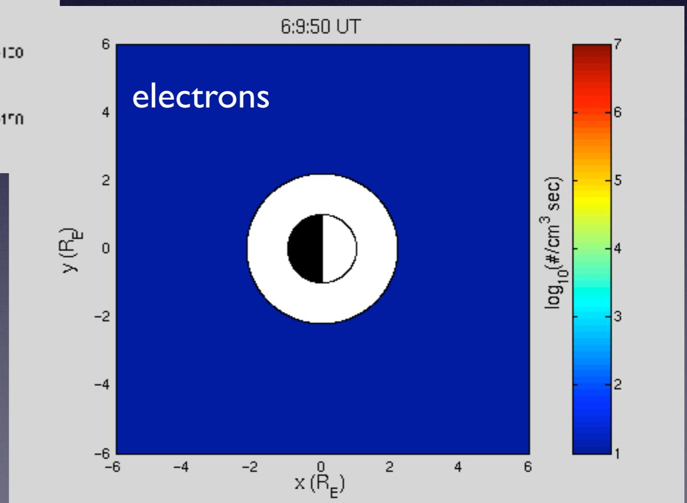
Test particle simulation shows how electrons move inward and gain energy
