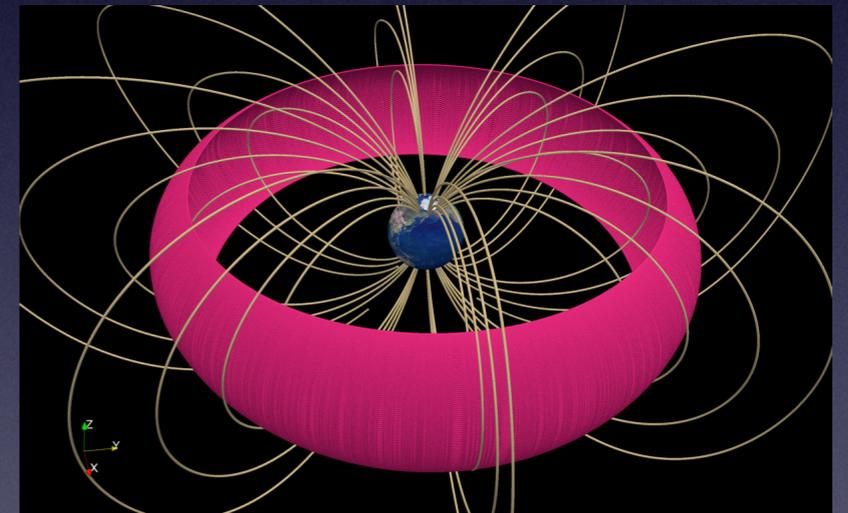
$$\mu = \frac{p_{\perp}^2}{2mB} \quad J = \oint p_{\parallel} ds = pI; \quad I = \oint \sqrt{1 - \frac{B(s)}{B_m}} ds \quad \Phi = \oint \mathbf{A} \cdot d\mathbf{l}$$
