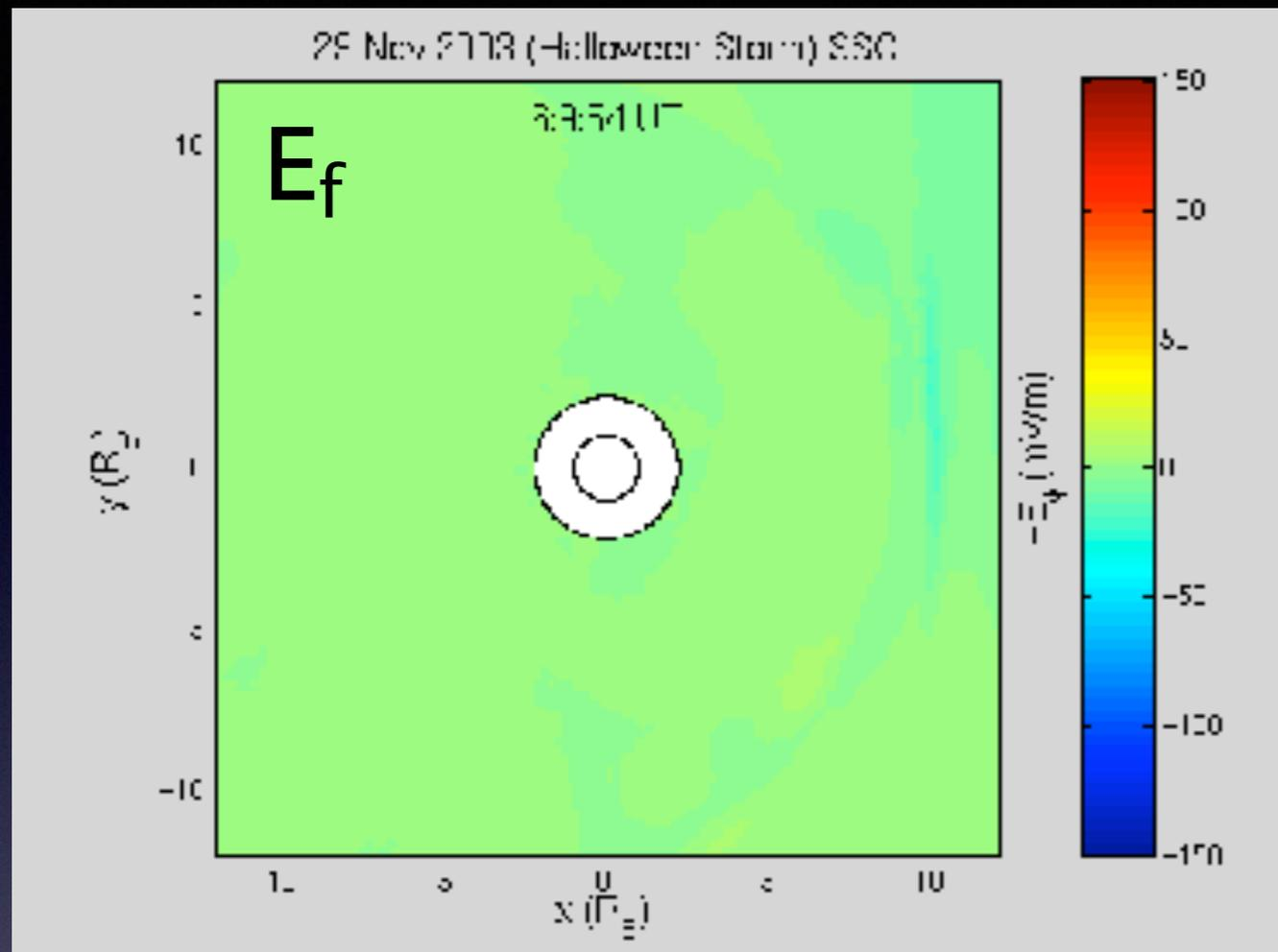
Electric field due to compression of magnetic field by solar wind
